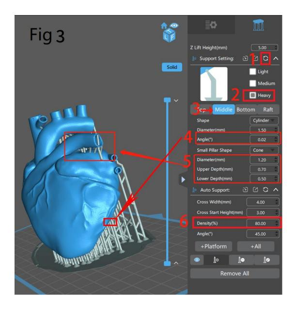
III. **Printing Settings:** You can download the resin printing parameters from RESIONE's official website. The detailed operations are as follows: RESIONE's official website —>Support —>Settings
