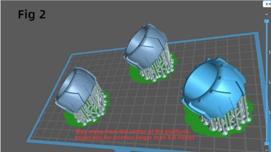
II. **Supports Settings:** Please use heavy and massive support (Density: 80%-95%), vertical supports (Angle: 0°). The supports in the middle of the model also need to be thick. (Figure 3). A thin raft or none raft are much better considering easy remove the prints from the build plate, because FX60 resin are very tightly stick to the build plate.
