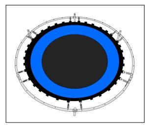
As shown in the picture, spring under heavy tension may require adjacent springs to be attached evenly, making the springs tension averagely distributed.
