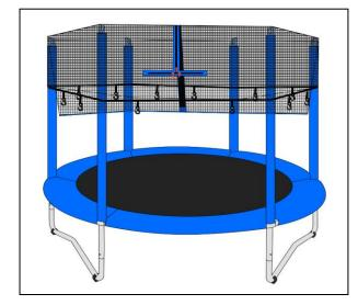
As shown in the picture, put the Safety Net (#6) on the 6 Upper Net Poles. Make sure the zipper is in the middle of the two Net Poles.
