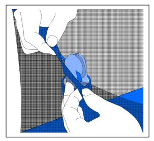
Clip the webbing on the top of the safety net into the tube cup.
