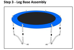
Insert Leg Base (#5) into Type T Connector (#4) as shown.
