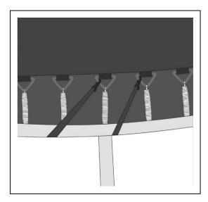
Then attach safety net mesh hooks to the nearest triangle ring of mat. **Do not attach to the springs.**
