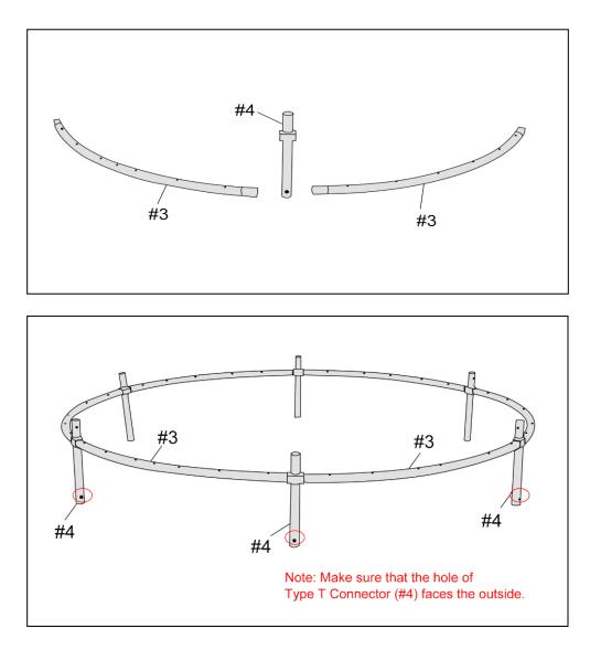
As shown in the picture above, assemble the frame of the trampoline.
