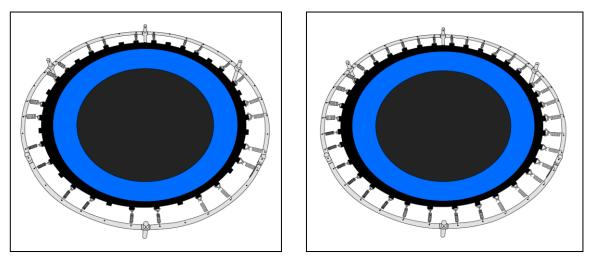
Refer to the picture to complete the assembly of the spring. If you notice that you have skipped a hole and v-ring connection, recount and remove or attach any spring required to maintain the count of springs. Attach the remaining springs until all the spring are placed on the frame and secured firmly.
