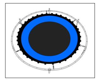
Use the spring loading tool (#9) to attach a spring (#6) with spring hooks face down to the v-ring of the mat and to the aligned hole of the trampoline frame. First assemble the 6 springs as shown in the picture. Drop hook into frame hole until it latches on completely and tap it down if hook is not completely in the hole.
