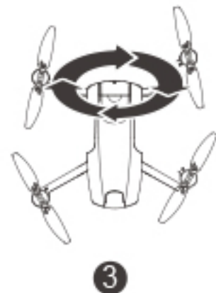
Hold the drone vertically and rotate 360 degrees for few times. Indicator flashes from rapidly to constant.
