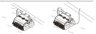
2. When pulling the cleaner out of the water, suspend the cleaner on the water for about 10-15 seconds to empty the water inside. Please hold the top handle only; never pull the cable.
