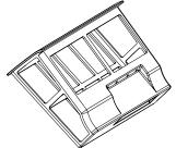
C. Re-install the filters, pay attention to the right position and slide the two clips to close the top cover.
