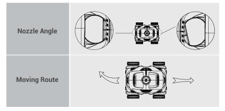
Setting Two: 0°--40°, when the cleaner does not have full coverage of the pool.
