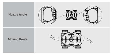
**Note:** These are recommended settings and different settings might apply to specific pools. So the operator can adjust the settings according to the principle of nozzle settings and the actual situation of the pool.
