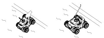
2. When pulling the cleaner out of the water, suspend the cleaner on the water for about 10-15 seconds to empty the water inside. Please hold the top handle only; never pull the cable.
