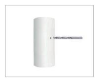
Drill a ¼" (6.5mm) hole on the drainpipe with an electric drill.
