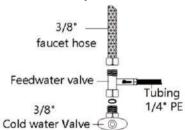
**Note:** Please check if the sealing ring is installed, or it may leakage.
