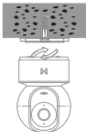
**⚠** When mounting the security camera on a wall: please note that the wall must be able to support at least triple the product's total weight.
