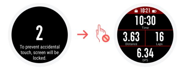
To prevent accidental taps and water interference with the touch screen, the watch automatically deactivates the touch screen function when a swimming workout begins. In such cases, you can control the workout with the watch buttons. After the workout ends, the watch reactivates the touch screen function.
