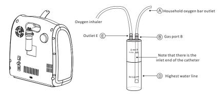
Put one end of the first conduit to the sump plug inlet port B (with the inlet conduit, as difference) A is inserted into the other end connected to the oxygen outlet household oxygen bar, and finally the end of the oxygen duct plug to the integrated water heater outlet E.
