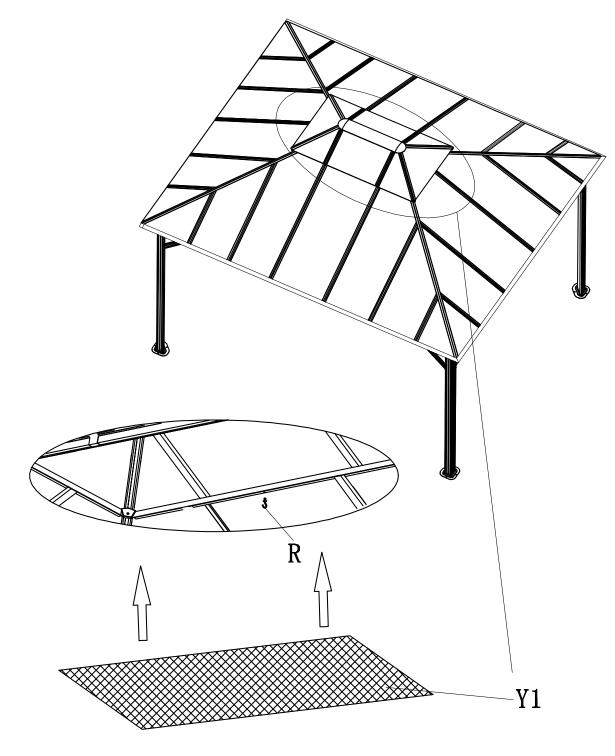
Put the small gauze net flat to the bottom of the top frame through Velcro, and install the lamp hook.
