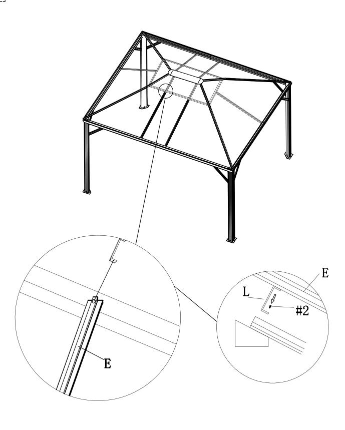
Use bolts(#2) through the hole at the bottom of C-type(L) and the one end of the middle tube, fixed to the hole on the top of the top frame(Q) and the other end over the beam. In addition, the two short-side installations do not need to cross the C-type(L).
