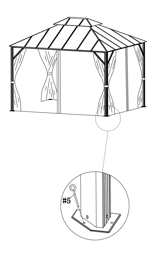
Use the stakes (#5) for ground fixing. Take note the anchoring devices to use may vary with ground status. Additional anchoring devices are not provided.
