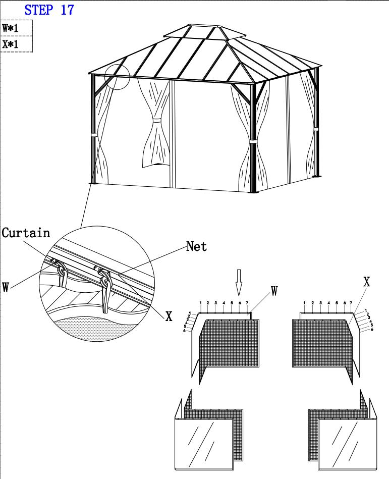
As shown in the figure, hang the cloth and gauze net through the hook on the guide rail.
