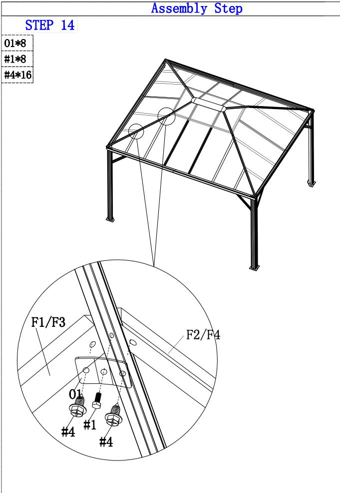
Install the three holes(01) on the two holes at the bottom of the pipe jacking(D) by bolts(#1). Then pass the screw (#4) through the holes on both sides of the three-hole plate (01) and secure it to the small holes on the top of (F1), (F2), (F3), (F4).
