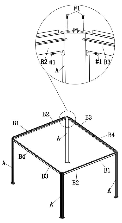
As shown, fix the crossbars assembly (B1)/(B2) and (B3)/(B4) to posts (A) by using bolts (#1).
