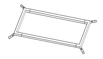
Assemble the top frames (Q) and (Q2) and secure them through the bolts (#1).
