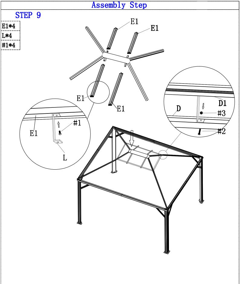
Place the small top of the previous step on the large top installed in step 7, place the bottom hole of the four C-type(L) installed on the small top on the first hole of the two holes of the top pipe(D), remove the bolt(#2) and the nut(#3) installed in the first step, and bolts(#2) the nut(#3) through the bottom hole of the C type(L) and the first top hole of the header(D). As in step 8, insert (E1) into the remaining tube of the top and install another C-type(L).
