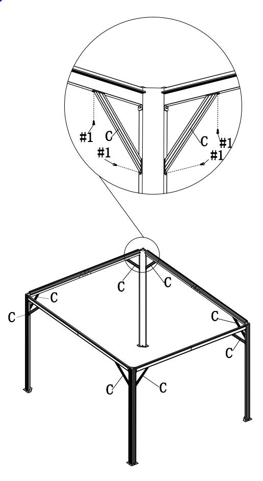
As shown, fix the braces (C) to posts (A) and crossbars assembly (B1)/(B2) and (B3)/(B4) by using bolts (#1).
