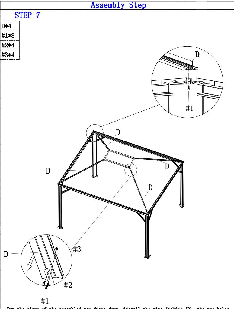
Put the claws of the assembled top frame down, install the pipe jacking (D), the two holes, the top two hole, the first hole through the bolts (#2) through the lower waist and the nut(#3), the second hole with bolts (#1), fix the four corners, rectangular top box and the top post (A), and fixed with bolts (#1).
