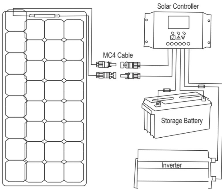
**Solar Controller, Alligator Clip and Storage Battery are not included in the package.**
