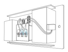
Ensure that the Chime Kit and wires DO NOT interfere with the mechanical parts of the chime. Mount on the outside of the chime if there is not enough room to mount inside. And replace your chime's cover.
