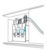
Locate the Chime Kit included in the smart doorbell's packaging, and the terminals on the inside of the chime. Connect one of the Chime Kit's prongs to the transformer terminal(usually labeled TRANS, T, AC, or 0). Connect the other prong to the chime's front terminal (usually labeled FRONT, F, 1, or C1). Either prong on the Chime Kit can be connected to either of the terminals on the chime.
