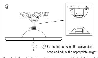
Hang the ball head at the top of the lamp body boom into the fixing bracket, connect the power cord, adjust the balance of the lamp body, and then clip the ceiling box to the fixing screw at the bottom of the fixing bracket, and tighten the screw.
