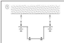
Take out the ceiling box and fixing bracket, fix the hanger on the ceiling, and tighten the screws to ensure safety and firmness.
