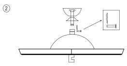
Take out the boom, put the ceiling box and the horn-shaped cover inside the boom as shown in the picture, then put the boom into the lamp body interface, insert the bolt horizontally, and then insert the safety buckle into the small hole on the bolt, And finally tighten the fixing screws of the boom.
