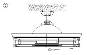
Finally, connect the lead wire of the product to the power cord, pass the whole lamp through the full screw, and fix it with a flat nut, the installation is complete.
