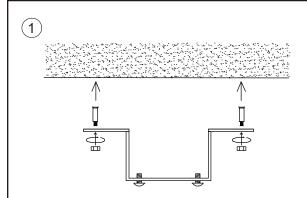
Take out the ceiling box and fixing bracket, fix the hanger on the ceiling, and tighten the screws to ensure safety and firmness.
