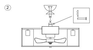
First, Take out the boom, put the ceiling box and the horn-shaped cover inside the boom as shown in the picture. Then, put the boom into the lamp body interface, insert the bolt horizontally, and then insert the safety buckle into the small hole on the bolt. Finally, tighten the fixing screws of the boom.
