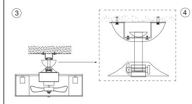
Hang the ball head at the top of the lamp body boom into the fixing bracket, connect the power cord, adjust the balance of the lamp body, and then clip the ceiling box to the fixing screw at the bottom of the fixing bracket, and tighten the screw.
