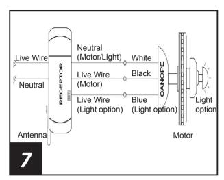
Respectively plug the wires of fan and light into receiver. (Light is optional.)
