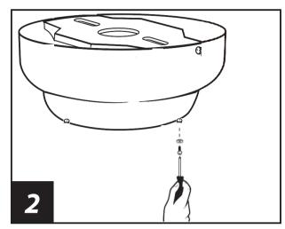
Remove the screw and washer from the two mating holes on the canopy. Loosen (do not remove) the screws in the mating slots on the canopy. Rototate the mounting bracket and remove it.
