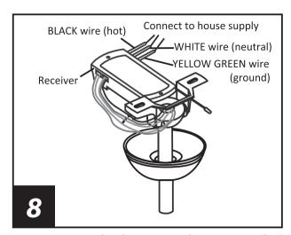
Insert receiver into bracket. Connect the BLACK wire (hot) to the BLACK wire marked "AC in L" from receiver. Connect the WHITE wire (neutral) to the WHITE wire marked "AC in N" from receiver. If there is a GROUND wire, connect it to the YELLOW GREEN wire from receiver.
