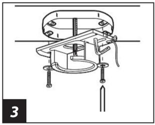
Securely screw the mounting bracket to the ceiling. For suspended ceiling wooden screws lock the bracket to ceiling joist (thickness > 30mm) directly. For cement ceiling, drill holes (M8 Depth40) and lock the bracket with explosion screws. The ceiling and bracket should be able to hold the weight at least 30kg.
