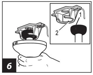
Carefully lift fan assembly onto mounting bracket. Rotate fan fully until notch on downrod ball (1) engages the ridge on the mounting bracket (2).
