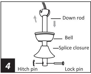
Remove the hitch pin and lock pin from the down rod. Slide the bell and splice closure off the down rod. Thread electrical wires through down rod.
