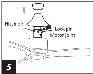
Insert the down rod into motor joint. Align holes and insert hitch pin and lock pin. Tighten yoke set screw securely. Slide the splice closure to the top of motor.
