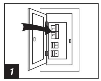
Unpack and inspect fan carefully to be certain all contents are included. Turn off power at fuse box to avoid possible electrical shock.
