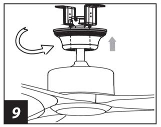
Raise canopy to bracket and align slotted holes in canopy with loosened screws in bracket. Twist canopy to lock and secure all screws.
