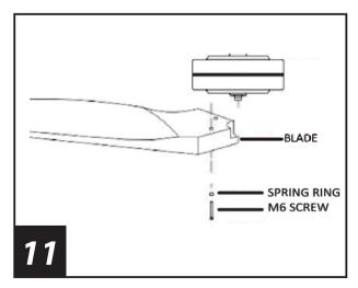
Thread the M6 screws with spring through holes end with blades.
