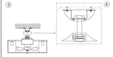
Hang the ball head at the top of the lamp body boom into the fixing bracket, connect the power cord, adjust the balance of the lamp body, and then clip the ceiling box to the fixing screw at the bottom of the fixing bracket, and tighten the screw.
