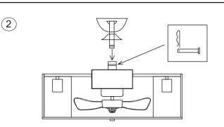
First, Take out the boom, put the ceiling box and the horn-shaped cover inside the boom as shown in the picture. Then, put the boom into the lamp body interface, insert the bolt horizontally, and then insert the safety buckle into the small hole on the bolt. Finally, tighten the fixing screws of the boom.
