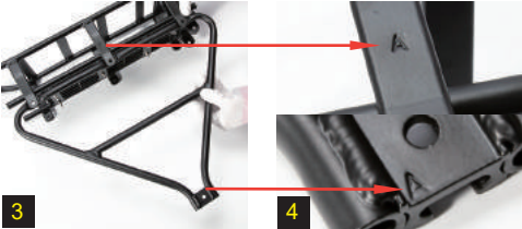
Photo 3,4: Assemble the rear rack construction (Please find the remark A to find the right direction)
