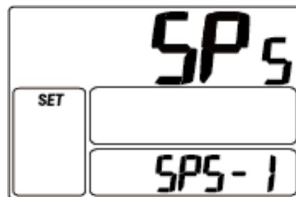
4.2.2 sensor orientation setting (B: anticlockwise F: clockwise) .
