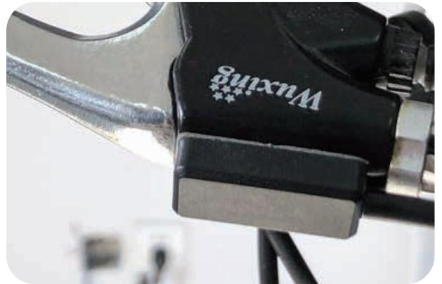
1: Remove the 3M tape on the sensor and stick on the brake lever as photo (position can be adjustable)
