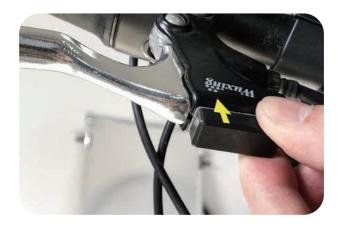
1:Remove the 3M tape on the sensor and stick on the brake lever as photo (position can be adjustable)
