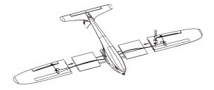
Assemble the wing to the body, tighten the screw to lock the wing. 安装机翼,固定管夹螺丝锁定机翼。
