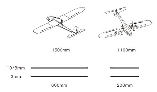
If user want use 1100wing span, the wing carbon tube need change 200mm. 若用户想使用1100mm翼展,需将机翼中间碳管切换至200mm.
