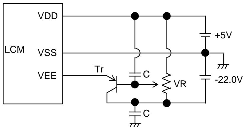
Note 1:  $C$  :  $3.3 \mu F$  (aluminum electrolytic capacitor)
