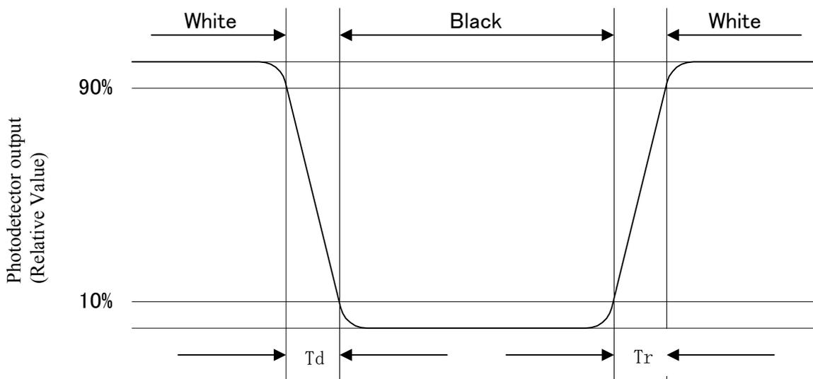
【Note4】 This shall be measured at center of the screen.
