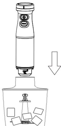
6) Lower the hand-held blender into food. Then press and hold the low speed button or high speed button to start operating.
