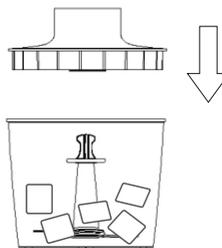
5) Insert the motor unit into the hole of the chopper lid.
