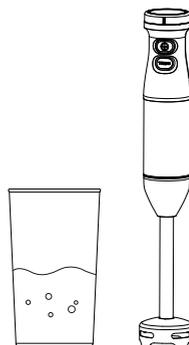
**Note:** There is a stepless speed knob, you can turn clockwise to increase speed, and turn anticlockwise to decrease speed. The speed knob is effective only after you pressing low speed button, once you pressed high speed knob, the speed knob is ineffective.
