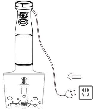
9) Then remove the motor unit from the chopper lid by turning it in anti-clockwise.
