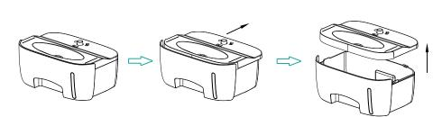
4. After pouring off the water, please put the water tank and water tank cover together.
