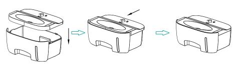
5. Then please put the water tank back in place. Press the power button, the machine will function again.
