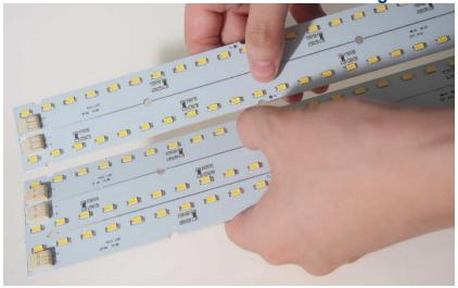
2. **Locate the terminal blocks on the module**. YUJILEDS® LED module has WAGO 2060 2-pole terminal blocks on both ends. The module can be powered from either side.
