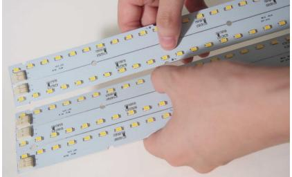
2. Locate the terminal blocks on the module. YUJILEDS<sup>®</sup> LED module has WAGO 2060 2pole terminal blocks on both ends. The module can be powered from either side.
