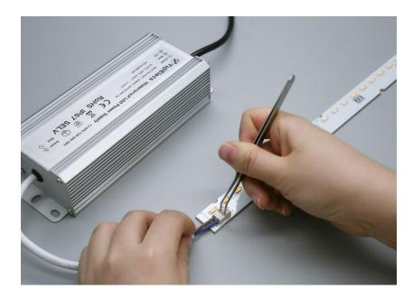
5. Release the push buttons and gently pull the wires to ensure they are securely placed.
