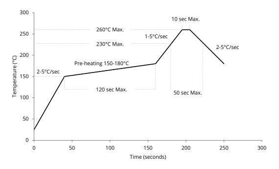
Note: Soldering paste with the melting point at 230  $^{\circ}\text{C}$  is recommended.
