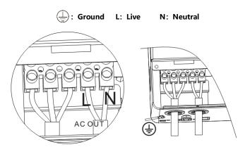
**Note:** The grounding wire shall be as thick as possible (cross-sectional area is not less than 4mm<sup>2</sup>). The grounding point shall be as close as possible to the all-in-one solar charge inverter. The shorter the grounding wire, the better.
