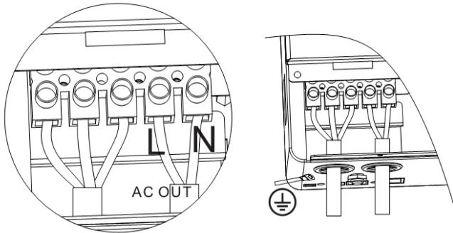
**Note:** The grounding wire shall be as thick as possible (cross-sectional area is not less than  $4\text{mm}^2$ ). The grounding point shall be as close as possible to the solar charge inverter. The shorter the grounding wire, the better.
