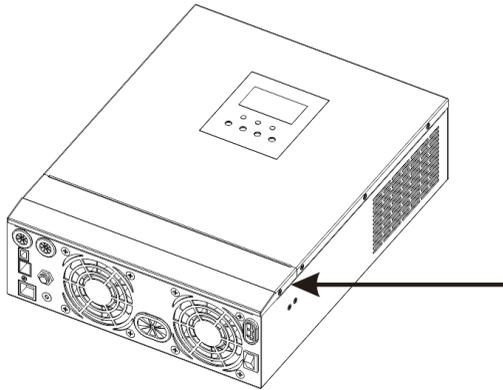
**Step 6:** Turn on the solar charge inverter
