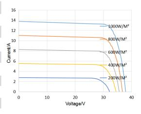
\*STC condition: 1000 W/m²,1.5AM and 25  $^\circ\!\!\mathbb{C}$  cell temperature.
