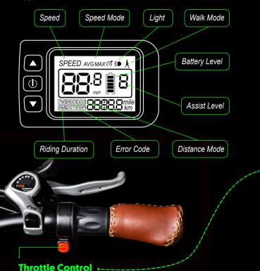
Twist n Go Throttle, to engage the throttle press the red button located below the gear lever this will enable the Navigata to move independent of any peddling and press again to disengage (if not used before we suggest to familiarise yourself with this function on open ground before use on main carriage way)
