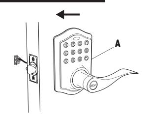
Check that the rubber gasket is secured on the exterior assembly. Place the exterior assembly onto the door with the tail piece going through the latch assembly. Route the control wire through the door over the latch assembly.
