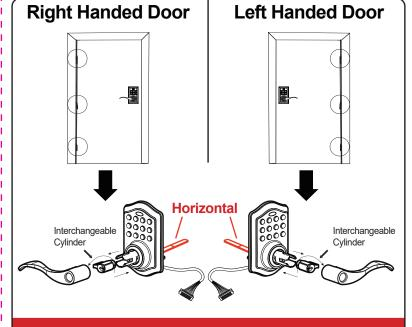
Reminder: Tail piece must be in the horizontal position only when removing or installing handles.
