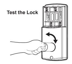
Check the Lock/Unlock function and that the Lever fully retracts the Latch.
