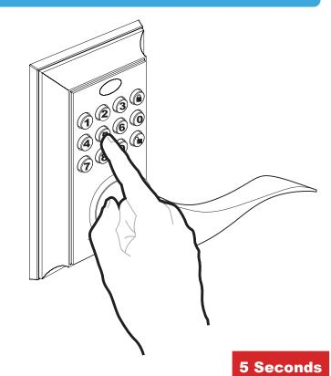
During programming, if there are no inputs for 5 seconds, the programming will exit and fail to complete.
