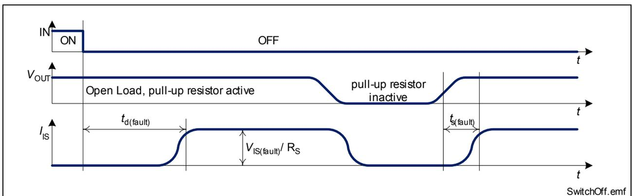
**Figure 16** Timing of Diagnosis Signal in OFF-state
