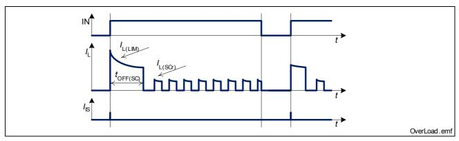
Figure 11 Shut Down by Over-Temperature
