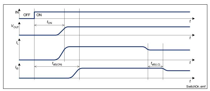
Figure 15 Timing of Diagnosis Signal in ON-state
