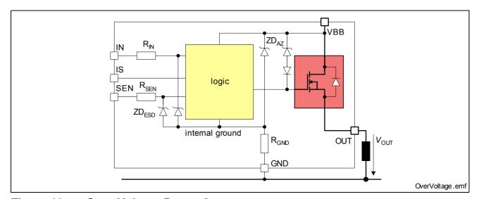
Figure 12 Over-Voltage Protection
