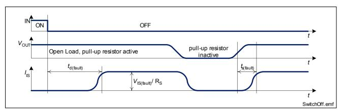
Figure 16 Timing of Diagnosis Signal in OFF-state
