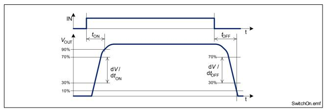
Figure 6 Switching a Load (resistive)
