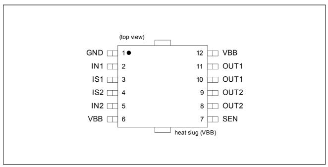
Figure 3 Pin Configuration P-DSO-12-2
