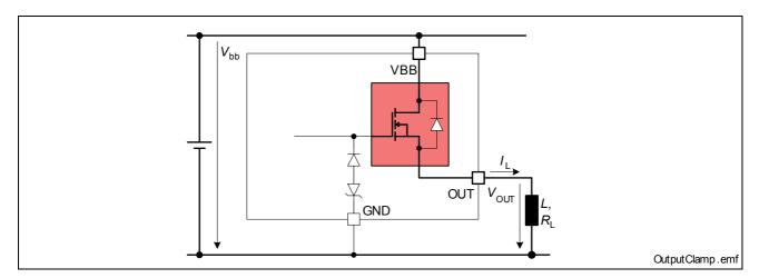
Figure 7 Output Clamp (OUT1 and OUT2)
