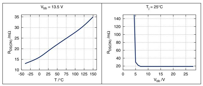
Figure 4 Typical On-State Resistance
