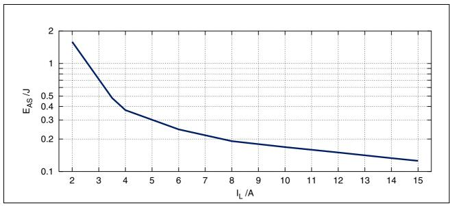
Figure 9 Maximum energy dissipation single pulse,  $T_{i,Start} = 150$ °C
