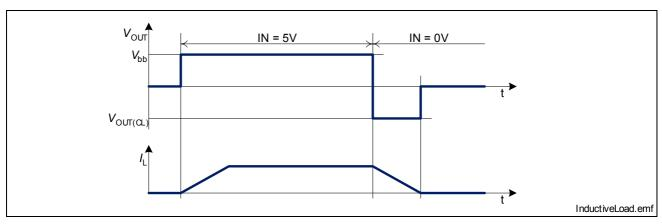
Figure 8 Switching an Inductance
