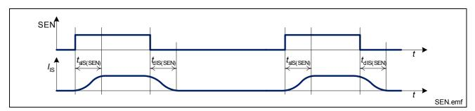
Figure 17 Timing of Sense Enable Signal
