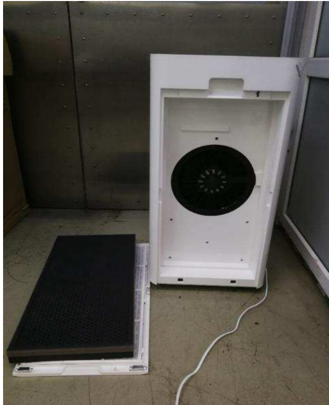
Photo 7 - Cover open and filter removed
