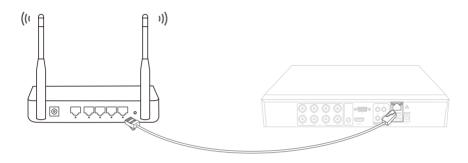
4 Connect the AHD camera with the 2-in-1 Video/Power Cable.
