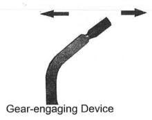
If there is gear-engaging device in your kart, you must make clear the function and operating ways of each gear so that you can avoid the danger arising from the unexpected running.
