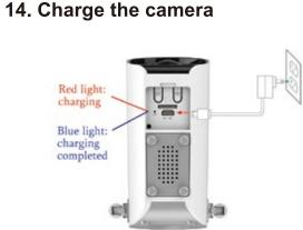
Remove the 5V1A power adapter and align the USB icon to insert the USB port **14.1** When the power adapter is connected to the USB port, you will see the red light **14.2** When the power is 100%, you can see the blue
