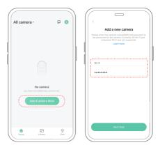
To ensure a longer distance connection, the camera only supports the 2.4Ghz Wi-Fi with stronger wall penetration capability and does not support Wi-Fi for enterprise-level authentication currently. Please ensure that the entered Wi-Fi meets the requirements. After completion, click "Continue" to generate the QR code for pairing the camera.
