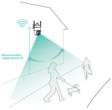
For outdoor use, please install the camera upside down to maximize the waterproof performance and the human body infrared sensor's effectivity.
