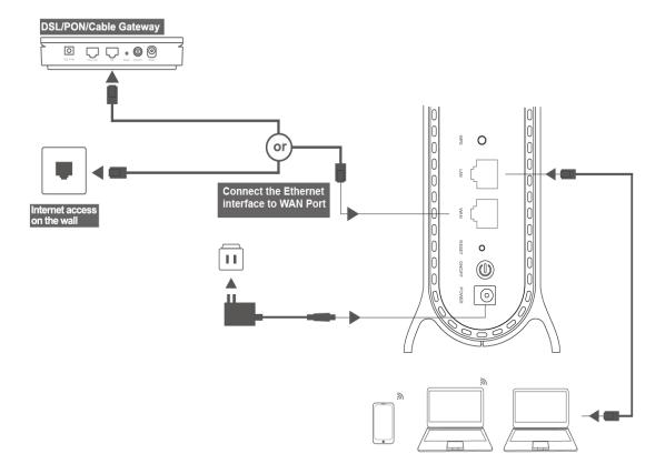
The Azores Router can be connected according to the diagram above.
