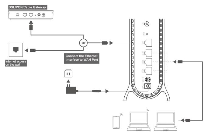
The Azores Router can be connected according to the diagram above.
