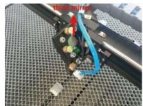
The mirrors can be cleaned in place using a lens-cleaning tissue or cloth or they can be removed by turning them counterclockwise. Take care not to touch the surface of the mirrors directly. Avoid pressing hard enough to grind any debris and cause a scratch. If the mirrors are removed for cleaning, reinstall them by turning them into place clockwise while being careful to avoid any scratches.
