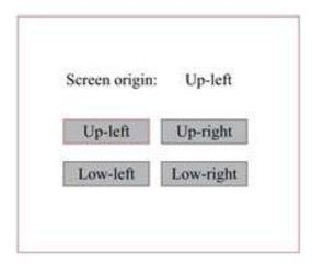
This interface shows the position of the origin. Different origin positions can generate different reflections of the graph over the X/Y axis. The operation method is the same as described above.
