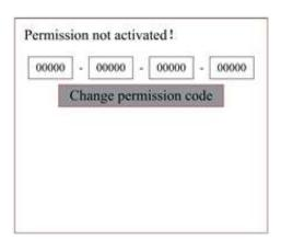
Press ENT once to select the first field, and press ENT a second time to bring up the keyboard.
