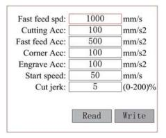
Select and adjust the parameters by pushing the arrows. When you finish your adjustments, move the cursor to Write and press **ENT** to save the parameter change or **ESC** to exit without saving. Read can load saved parameters.
