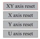
Push  $\triangle$  or  $\nabla$  to select an item. Press **ENT** to start the resetting of the selected axis, and the message "Resetting Is Underway" will show on the screen. Upon completion, the message will automatically disappear and the system will return to the main interface.
