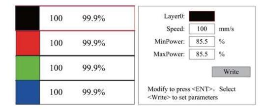
The red cursor will be on "Layer" by default. Push the ◀ and ▶ keys to select the intended layer. Move the cursor to Write and press **ENT** to save the parameter change or **ESC** to exit without saving. The operation method is the same as that of the max/min power setting.
