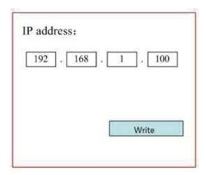
Push  $\triangleleft$  or  $\triangleright$  and  $\triangle$  or  $\blacktriangledown$  and ENT keys to change the parameters. When you finish your adjustments, save them by selecting Write with the ENT key or hit ESC to leave without saving your changes. Read can load saved parameters.
