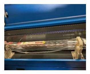
You will need to place a piece of tape at each stage of the laser path, marking it to confirm that that stage remains correctly aligned. When it is not, you will use the laser tube's brackets or the screws on the back of the misaligned mirror to correct the problem. Once the provided tape runs out, we recommend masking tape as it is easy to manage and use.
