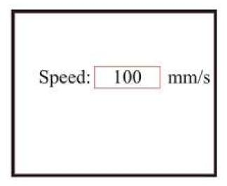
Push the ▲ and ▼ keys to change the parameter value. Press ENT to save the change. Press ESC to invalidate the change and return to the main interface.
