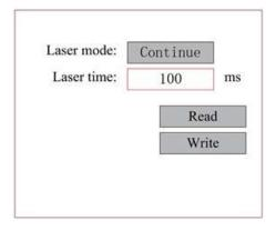
The operation method is the same as the previous setting. When Continue is selected, press **PULSE** to fire the laser, and release the key to finish firing. When you finish your adjustments, save them by selecting Write with the **ENT** key or hit **ESC** to leave without saving your changes. Read can load saved parameters.
