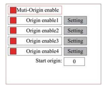
Press **FN** to select an item. When Multi Origin Enable is selected, press **ENT** to enable or disable the item. When enabled, the small box will be red and, when disabled, the small box will be grey. When selecting Set Origin or Next Origin, push ◀ or ► to select the value. When changing the parameters of Set Origin, remember to press **ENT** to validate the change. Parameters will be saved automatically when the interface is closed.
