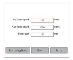
Select and adjust the parameters by pushing the arrows. When you finish your adjustments, move the cursor to Write and press **ENT** to save the parameter change or **ESC** to exit without saving. Read can load saved parameters. Start cutting frame will cut the frame according to the current parameters.
