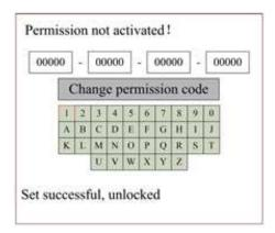
Use the direction keys and **ENT** to select the correct character. Press **ESC** and then **ENT** to re-enter a field if you make any mistakes. Use the arrow keys to move to the other entry fields, and enter their contents in the same way. After all fields are correctly entered, select Change Permission Code and press **ENT** to leave this screen and return to the main menu.
