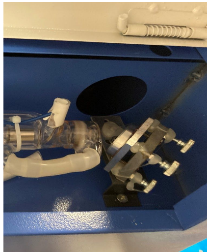
Fig. 4-3 - Adjustment Set Screws Behind the First Mirror
