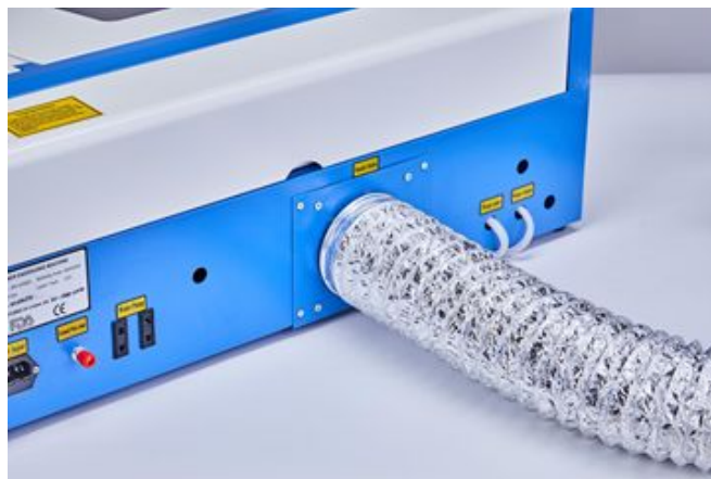
Fig. 2-2 - Exhaust Pipe Connection
