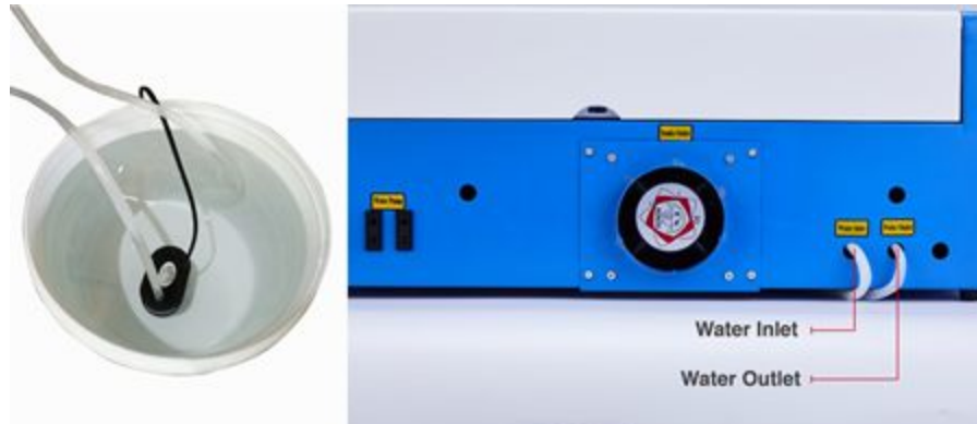
Fig. 2-1 - The Cooling Water System
