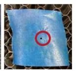
When the laser is well centered along the entire path from the tube to the workbed, your laser mirrors are all correctly calibrated and (assuming they are clean) performing at optimum efficiency.
