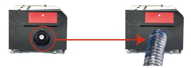
The other end should be connected to a dedicated purifier or (if the fumes are not hazardous and meet local and national air safety standards) placed out a window. **NEVER** operate the laser if the vent is not purifying or removing the fumes produced by the target material. Research materials before use and never operate the laser on any (such as PVC, teflon, and other halogen-containing substances) that can produce corrosive, hazardous, or even deadly fumes.
