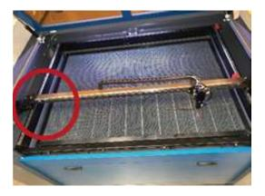
Once set, place another piece of tape on the 2nd mirror's frame. **DO NOT** place the tape directly onto the mirror. Repeat the steps from §5.4.1 and, if necessary, adjust the set screws on the 1st mirror. Test again until the beam is well aligned and retighten the nuts on the set screws.
