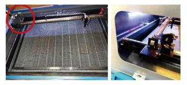
Once set, place a piece of tape on the 2nd mirror's frame. **DO NOT** place the tape directly onto the mirror. Repeat the steps from §5.4.1. If the laser is not centered on the 2nd mirror, you will need to adjust the 1st mirror's set screws accordingly.
