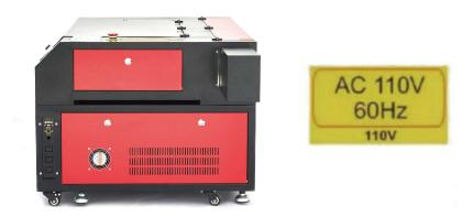
Fluxuation along the line should be less than 5%. If this is exceeded, the fuses will blow. They are located in the connection socket and are accessible from the exterior. Similarly, do not connect this device to standard extension cords or power strips. Connect it directly to a grounded outlet or use a surge protector rated over 2000J.
