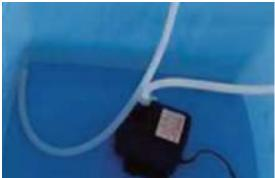
Connect the water pump to its power supply. For best results, use an power outlet on a separate fuse from the engraver itself. If no such outlet is available, the pump can also be plugged into a dedicated socket located on the side of the engraving cabinet. Once the pump is plugged in, water should begin to run through your machine and back into your tank. **ALWAYS** obtain visual confirmation that the water is flowing through the laser tube before starting your laser.
