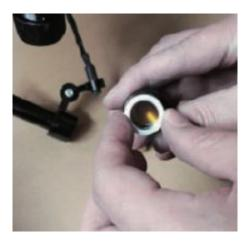
4. Remove the pressurized air hose and laser guide connections.
