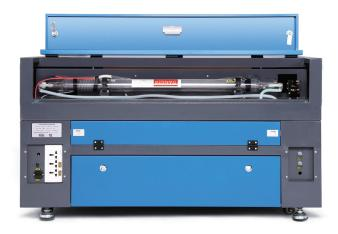
**Step 4.** Inside the main bay, remove the nylon cable ties from the X axis and the honeycomb table.
