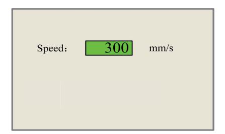
A cursor will appear when pushing  $\leftarrow$  or  $\rightarrow$ . Move the cursor to the numeral area and push  $\triangle$  or  $\nabla$  to change the value. Press **ENTER** to save the change. Press **ESC** to invalidate the change and return to the main interface.
