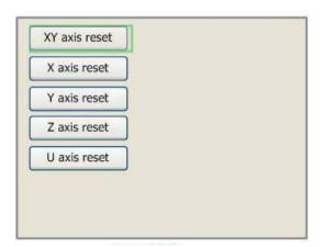
Push  $\triangle$  or  $\nabla$  to select an item. Press **ENTER** to start the resetting of the selected axis, and the message "Resetting Is Underway" will show on the screen. Upon completion, the message will automatically disappear and the system will return to the main interface.
