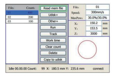
The system will automatically read the memory files. The file name and the work times will be listed and the selected file will be previewed in the upper right corner. Different memory files can be selected by using  $\blacktriangle$  or  $\blacktriangledown$ . Press **ENTER** to preview the selected file on the main interface. Press **ESC** to close the preview.
