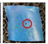
When the laser is well centered along the entire path from the tube to the workbed, your laser mirrors are all correctly calibrated and (assuming they are clean) performing at optimum efficiency.
