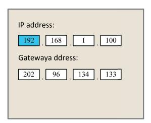
Press Z/U to select an item, and push ← or → and ▲ or ▼ to change the parameters. Press ENTER to save the changes or ESC to discard changes and return to the previous menu.
