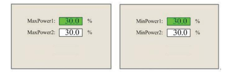
When  $\mathbb{Z}/\mathbb{U}$  is pushed, the green block can move up and down to denote the changing item. Then  $\triangle$  or  $\nabla$  and  $\leftarrow$  or  $\Rightarrow$  can be used to change the value. Press **ENTER** to save the change. Press **ESC** to invalidate the change and return to the main interface.
