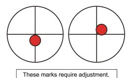
The laser mark should be near the center of the hole. If the laser is not centered on the 1st mirror, cut the power to your laser and carefully adjust the laser tube on its brackets. This may require loosening the screws on its stand and adjusting its brace wheel. Be careful not to over loosen the screws and not to overtighten them. Only adjust one stand at a time.
