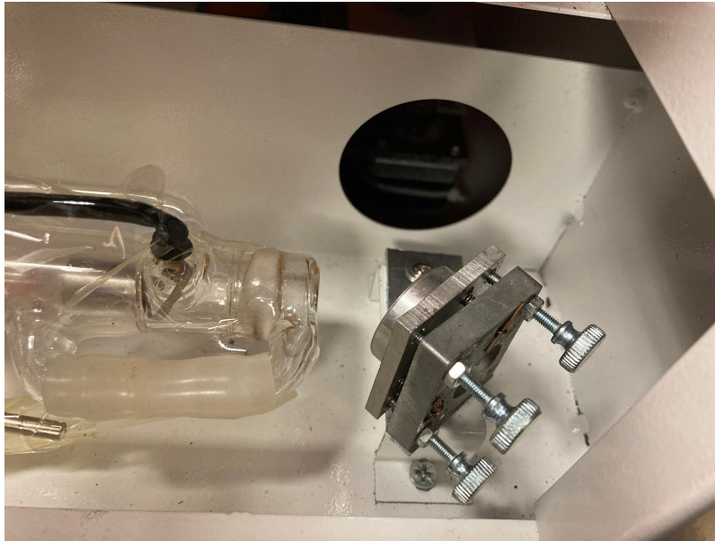
Fig. 4-3 - Adjustment Set Screws Behind the First Mirror
